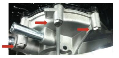
7a. Using a 1/4" allen wrench, mount the main bracket using the supplied .75" spacer and the 5/16-18 x 6.25" bolt through the bottom drivers side of the bracket and water pump. Tighten just enough to hold in place.
