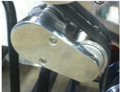
18. Install the A/C Manifold using a 6mm allen wrench on (2) M8 x 1.25 x 30mm SHCS. Be careful and make sure the o-rings are well seated. Inspect the A/C fit-tings, be sure the smaller diameter fitting is towards the rear of the vehicle.
