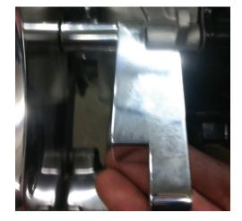
9. Install the rear AC bracket, the 1.5" spacer and 5/16-18 x 6.25" bolt through the passengers side main bracket and top passengers side water pump mounting location. Tighten just enough to hold in place.
