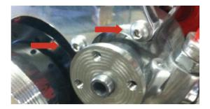
24. Using a 9/16" wrench, install the tensioner using the 3/8-16 x 2-1/2" hex head bolt with a small amount of blue Loctite on the threads and a 3/8" washer.
