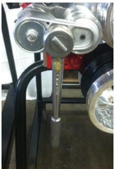
27. Using a 1/8" allen wrench, install the tensioner cover using the (2) 10-32 x .5" FHCS with a small amount of blue Loctite on the threads.
