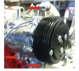
23. Using a 3/16" allen wrench, install the type II power steering pump with (2) M8 x 1.25 x
