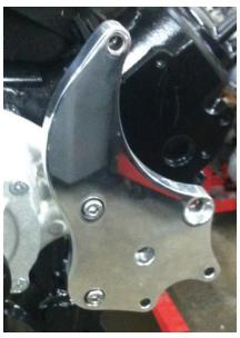
Install the alternator bracket, 1.6" spacer and m8-1.25 x 5.75" bolt through the drivers side bracket. Place some anti-seize on the threads. Tighten just enough to hold in place.
