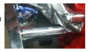
7b. Use the 3.230" spacer and 3/8-16 x 5" bolt through the bottom passengers side of the bracket and water pump. Tighten just enough to hold in place.
