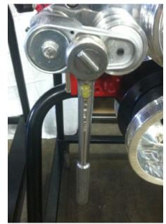
17. Using a 1/8" allen wrench, install the tensioner cover using the (2) 10-32 x .5" FHCS.
