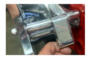
9b. Install the rear AC bracket (stepped bracket), the 1.853" spacer and 3/8-16 x 5" bolt through the passengers side main bracket and top passengers side water pump mounting location. Tighten just enough to hold in place.
