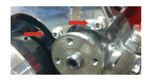
14. Using a 9/16" wrench, install the tensioner using the 3/8-16 x 2-1/2" hex head bolt.
