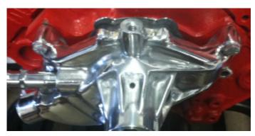
7a. Using a 5/16" allen wrench, mount the main bracket using the supplied 3.190" spacer and the 3/8-16 x 5" bolt through the bottom drivers side of the bracket and water pump. Tighten just enough to hold in place.
