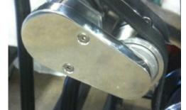
18. Install the cap on the alternator fan/pulley using a 1/16" allen wrench on the (2) 4-40 x 1/4" BHCS for the bolt on style or press on for the press fit style (shown).
